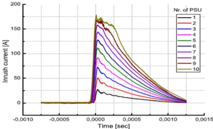
**Fig.5: Showing how inrush current increases as drivers are added to MCB**
