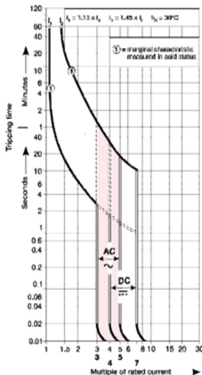
peak value and its time duration. Accordingly, an MCB could be tripped either by a high peak of short duration, or a lower peak of longer duration. In either case, the objective is to ensure that the MCB trips before passing excessive energy, yet does not trip and cause lighting blackouts when it does not need to. MCB manufacturers' solution to this is to offer a choice of trip characteristics in addition to their steady-state current rating;
